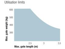
The shape, the height of the gate and the weather conditions can considerably reduce the values shown in the graph to the side. Use in windy areas 230Vac models.
