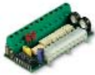
PIU expansion card for control unit
