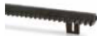
ROA6 M4 25x20x1000 mm slotted nylon rack with metal insert. For gates weighing up to 500 kg. Pc./Pack 10
