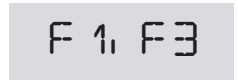
Three-phase connection R-S-T with reversed sequence (the control panel reverses automatically OPEN and CLOSE of the motor)
