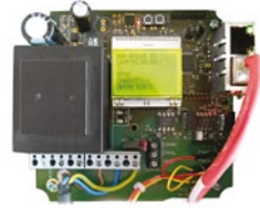
NDA008 K65 module for D-Pro Automatic control unit, for remote control (combined with NDA0006 module).
