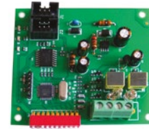
NDA070 K70 expansion module for D-Pro Automatic for 2 channels loop detector.
