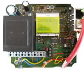
NDA008 Repeater module with integrated router.
