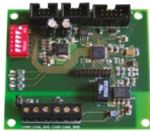
NDA006 K60 module for D-Pro Automatic control unit, to communicate via CAN bus (combined with NDA008 module).
