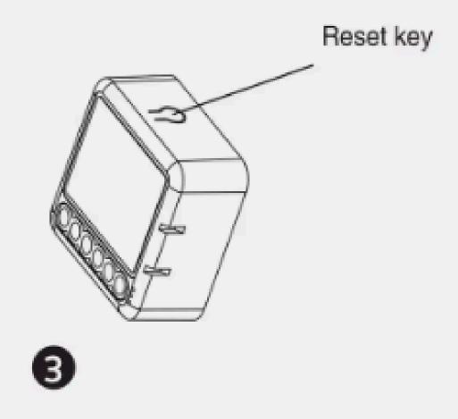
After the wiring of switch module is done, press the reset key for about 10 seconds until the indicator light inside the module is flashing quickly for pairing.
