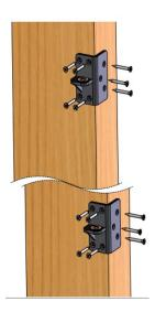
Step 5. Align the axes of the upper and bottom fixed inner brackets with the hinge holes on the gate post and install them.
