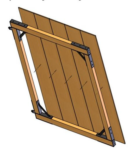
Step 4. Measure the gate frame to determine the hinge height, and tighten the flathead wood screws to fixed the gate hinges on the gate post.
