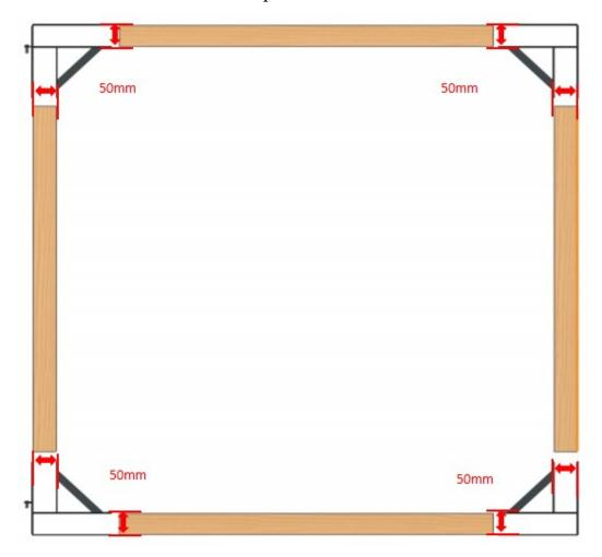
Step 2. Determine the position and tighten the flathead wood screws at the four brackets.
