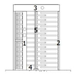
First, assemble the side railings 1 and 2. Then, place the top chassis 3 on top of 1 and 2 and tighten the fixing screws. Place the bottom bearing plate 4. Finally, place the 5 rotating shaft on the bottom bearing 4, connecting the upper part of the rotating shaft to the top chassis. Adjust accordingly.
