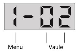
\* As shown in the figure above, it means that the current menu is "Open Mode", and parameter 02 means "open by left IR1 induction".
