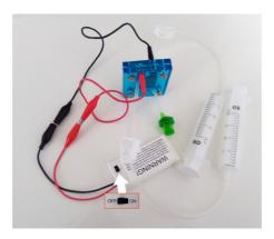
Connect the red & black lead cables to the fuel cell. During this process make sure the battery pack is turned off! Attach the red and black cables from the battery pack to the crocodile clips that are connected to the fuel cell (make sure the red and black leads do not touch eachother – this would create a short circuit!).
