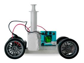
This car is powered by a zero emission fuel and it can with help from the included motor drive both forward and backward. Create your own car and race with other classmates who will drive longer distance on single "tank" of hydrogen. For this race you have to create your car as light as possible!
