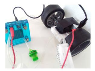
A fuel cell has both a negative (Hydrogen) and a positive (Oxygen) side. While using the fuel cell it is important to make sure the polarities (red to red & black to black) are correct as it will affect the direction of the motor. This means the car will drive backwards if you switch the polarity.
