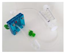
Attach a syringe to the top nozzle on each side of the fuel cell (these will be for gas storage).
