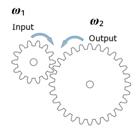
Because the diameter of the driver or input gear is smaller than the diameter of the driven or output gear, the angular speed of the driver gear  $\omega_1$  is greater than the angular velocity or driven gear  $\omega_2$
