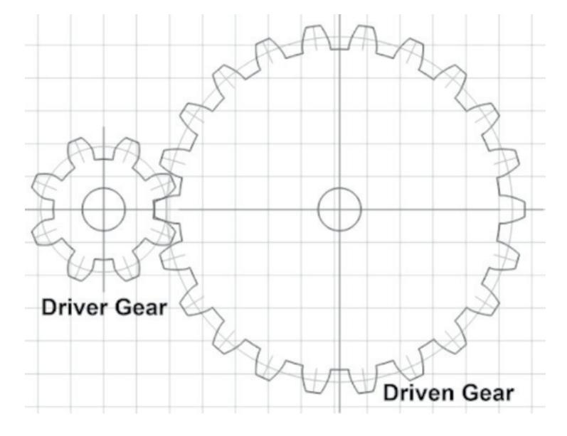
In a gear system, the gear connected to the power source is known as the **driver gear**, while the gear that delivers the output is called the **driven gear**.
