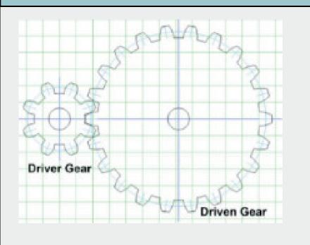
Lower overall speed Higher torque
