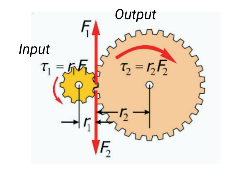
Torque of the input or driver gear  $\tau_1$  is less than the torque of the output or driven gear  $\tau_2$  because the input gear has a smaller diameter.
