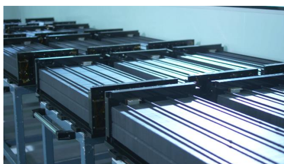
Fig. 7 Completed fuel cell stack without housing
