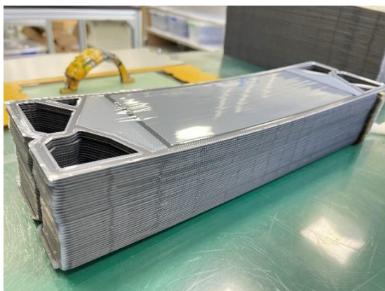
Fig. 4 Finished single cells, bipolar plate including MEA.
